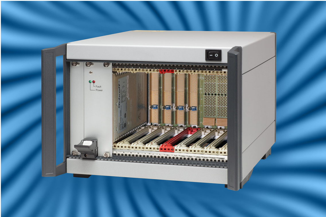
Sample CompactPCI® PlusIO Rack
