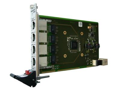
The G211 quad Ethernet interface is a rugged single Eurocard CompactPCI<sup>®</sup> Serial peripheral board. It can be used in combination with a CompactPCI<sup>®</sup> Serial or CompactPCI<sup>®</sup> PlusIO CPU board in a CompactPCI<sup>®</sup> Serial or hybrid system.
