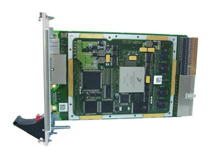
The F50P is a versatile, rugged PowerPC® based single-board computer for embedded applications. It is controlled by an MPC8548, or optionally an MPC8543 PowerPC® processor (alternatively with encryption unit) with clock frequencies between 800 MHz and 1.5 GHz. The SBC is equipped with ECC-controlled, soldered-on DDR2 RAM for data storage, with up to 16 GB of solid-state Flash disk for program storage as well as industrial FRAM and SRAM.
