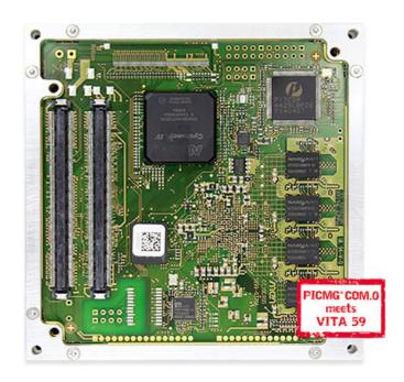
The CC10C is a Rugged COM Express® module (RCE) built around the Freescale™ ARM® i.MX 6 series of processors with a Cortex®-A9 architecture. Supporting different types of the i.MX 6Solo, 6DualLite, 6Dual and 6Quad families, the computer-on-module is widely scalable, e.g., to processing or graphics requirements. Where less performance is needed, you can optimize costs by choosing a single- or dual-core processor instead of a quad core.
