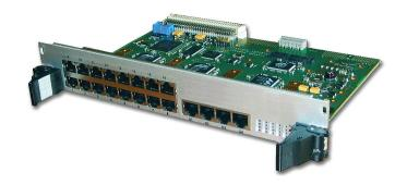
T3200b is a range of highly integrated Layer 2/3 Ethernet switches. The switching capability provides up to sixteen 10/100BT and eight 10/100/1000BT front Ethernet ports.
