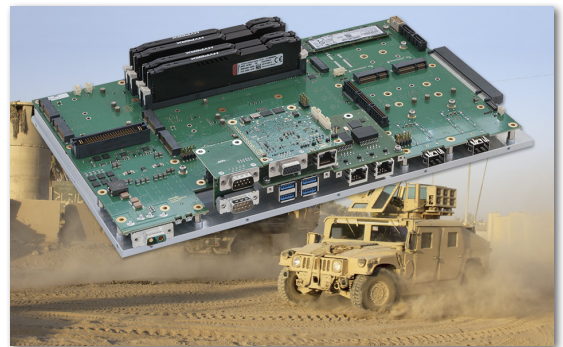
MXCS Open-frame solution used on military vehicle
