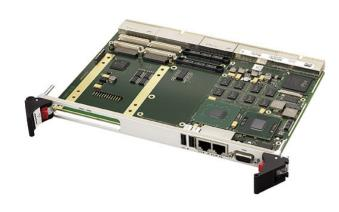
The D9 6U single-slot SBC supports a variety of Intel® Core<sup>™</sup> Duo and Core 2 Duo processors from the highend 2.16 GHz T7400 to the low-voltage dual-core versions down to a selection of Celeron® M types. It is designed especially for embedded systems which require high computing and graphics performance and low power consumption.
